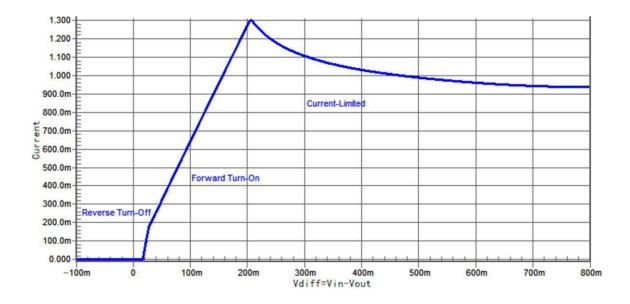
7.2 On-current and Dropout Voltage at 3V (test conditions: VI=3V)
